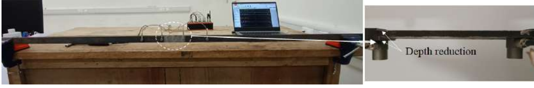
Figure 4.16: Experimental setup - damaged structure.
