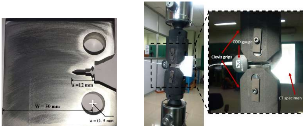
(a) The geometry of the CT specimen. (b) The experimental setup with a closed view of the specimen in hold with COD gauges.
